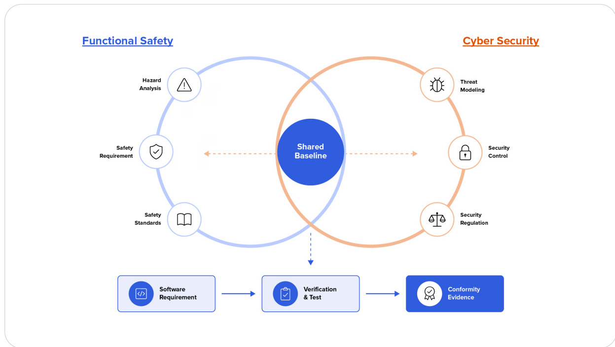
Figure 1: Hazard analysis and threat modeling converge on the same requirements baseline. The relationship between a safety obligation and the security control that protects it is recorded once, and visible whenever either one changes.
